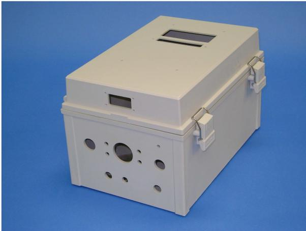
The complex and very tight tolerance hole pattern shown in the base was required to match with the existing sensor mounting configuration and also mate to an interior mounted chassis. This complex hole pattern is milled using specialized high spindle speed, CNC machinery. However, should production volumes increase, the option exists to modify the injection mold to
