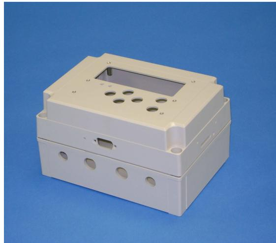
A precision set of 6 holes is drilled within the perimeter outline of the cover. Hole to hole spacing is maintained at a tight tolerance to match the tolerances of the PC board. A secondary manufacturing step is performed to press fit the 6 threaded metal standoffs which are specifically designed for plastic materials.
